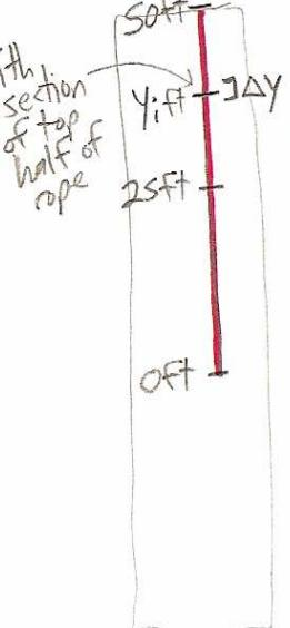
Let's focus first on the top half: The  $i$ th section of the top half weighs  $0.5 \frac{\text{lb}}{\text{ft}} \cdot \Delta y \text{ ft} = 0.5 \Delta y \text{ lb}$
