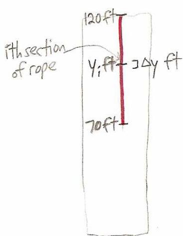
The  $i$ th section of rope weighs  $0.5 \frac{\text{lb}}{\text{ft}} \cdot \Delta y \text{ ft} = 0.5 \Delta y \text{ lb} = F_i$
