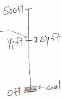
$$\text{Total work done} = W_1 + W_2, \quad \text{where } W_1 = \text{work done lifting the cable} \\ W_2 = \text{work done lifting the coal 500 ft.}$$
