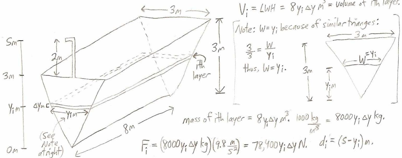
$$W_i = F_i d_i = 78,400(5y_i - y_i^2) \Delta y \text{ J. Total work } W = \lim_{n \rightarrow \infty} \sum_{i=1}^n 78,400(5y_i - y_i^2) \Delta y = (\text{next line})$$
