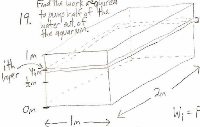
$$V_i = \text{volume of } i\text{th layer} = LWH = 2 \cdot 1 \cdot \Delta y = 2\Delta y \text{ m}^3. \\ \text{mass of } i\text{th layer} = 2\Delta y \text{ m}^3 \cdot 1000 \frac{\text{kg}}{\text{m}^3} = 2000\Delta y \text{ kg.} \\ F_i = \text{force required to raise } i\text{th layer} = (2000\Delta y \text{ kg})(9.8 \frac{\text{m}}{\text{s}^2}) = 19,600\Delta y \text{ N.} \\ d_i = \text{distance the } i\text{th layer must be raised} = (1 - y_i) \text{ m.}$$
