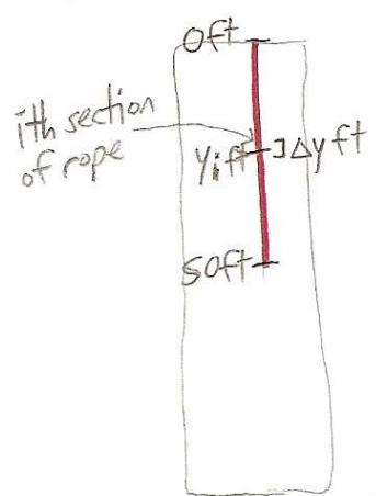
the  $i$ th section of rope weighs  $0.5 \frac{\text{lb}}{\text{ft}} \cdot \Delta y \text{ ft} = 0.5 \Delta y \text{ lb} = F_i$
